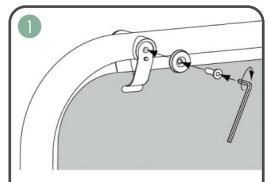
Slot panel on to the hanging clips. Attach the clips to the frame using the screw and fixings provided. N.B allen key under base.
