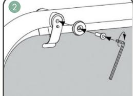
Place the curved fixing onto the frame followed by the hanging clip and the flat fixing. Screw all into place.
